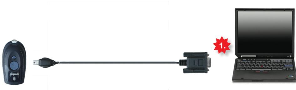
1. Connect serial cable with PC.
